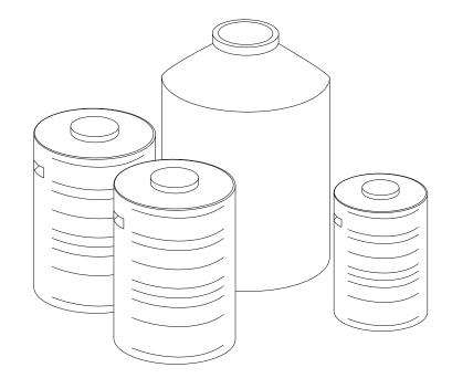
When urine cannot be used immediately or transported using a Conveyance technology (i.e., Jerrycans, see C.1), it can be stored onsite in containers or tanks. The storage tank must then be moved or emptied into another container for transport.
